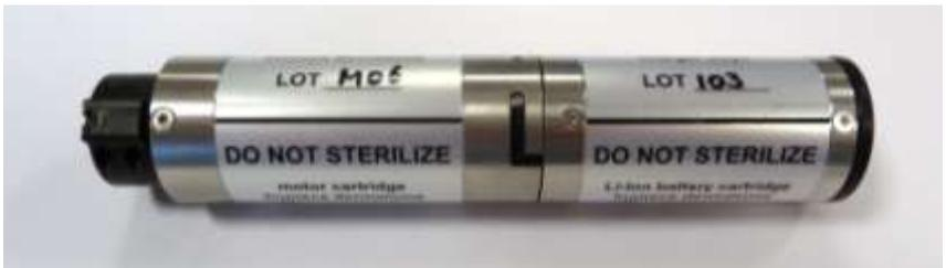
Fig. 4 Coupling of motor- and battery pack of a D42 dermatome
