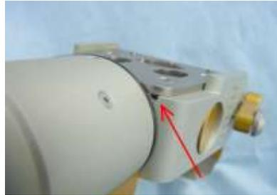
Fig. 3b Cavity for lifting covering plate
