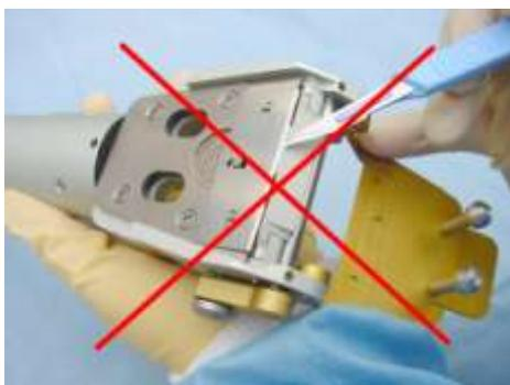
**Fig. 16** Wrong way to remove blade
