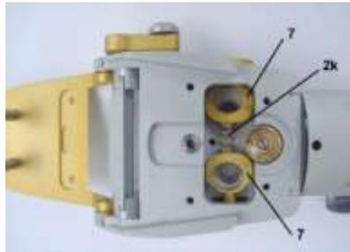
Fig. 3f Removing locking buttons
