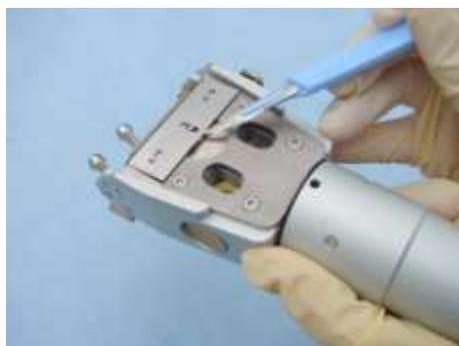
**Fig. 15** Right way to remove blade
