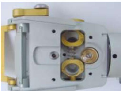
**Fig. 4 Correct orientation of the button rings and spring**
