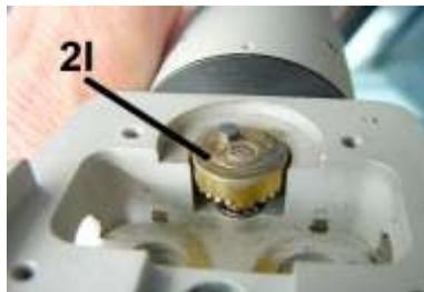
Fig. 3h Gearwheel to be cleaned
