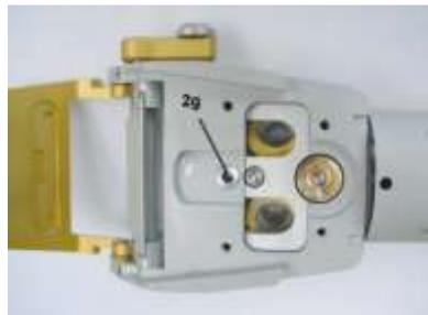
Fig. 3d Removing bearing
