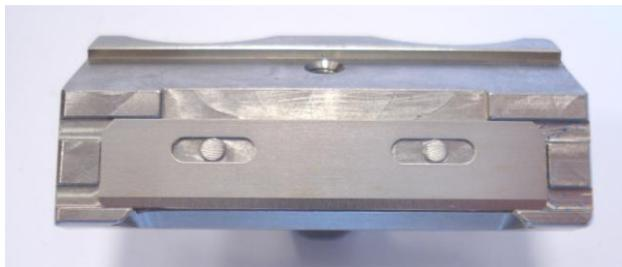
**Fig. 10** Correct position of the blade
