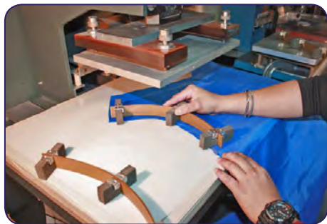
Custom fitting the RF sealing welds.
