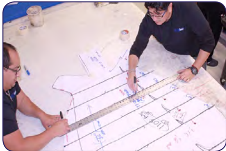
Measuring and drawing out the pattern based on your patients' unique measurements
